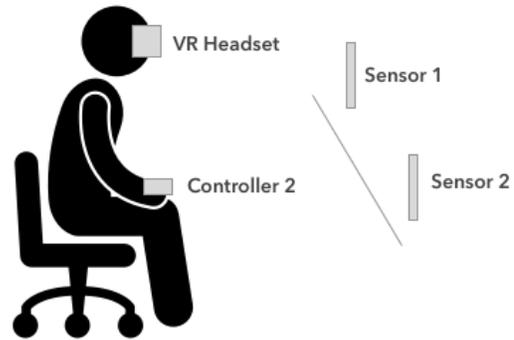
**Figure 1:** The figure depicts the experimental setup where the subject is made to sit in a rotating chair wearing the VR headset within the range of the VR sensors.
